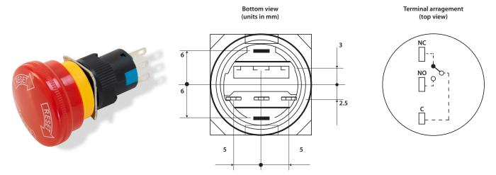
E-stop1 is an emergency (latching) stop pushbutton for 16 mm mounting hole. It's rated IP54 where seal is in place (seal included).
